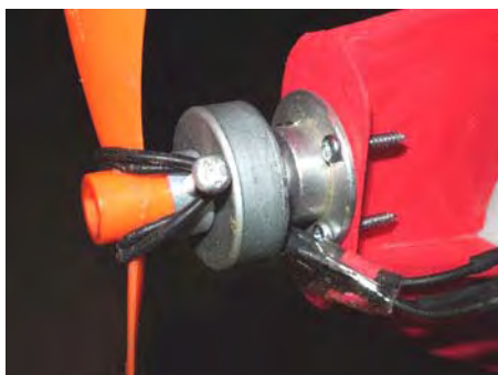
A 50 Watt CD ROM- based motor was used on the prototype
