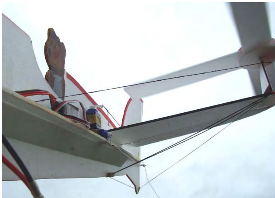
Rearwards view showing a fuselage sidepiece and 45 degree stiffener.
